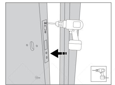
Install the handles on both sides of the lock and finally tighten the bottom with screws.
