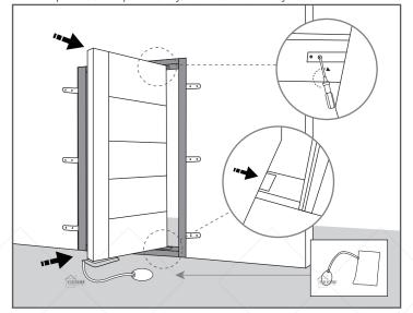
Install the door lock, measure with a ruler, draw the inside and outside positions of the lock handle with a pencil, and use an electric drill to drill out the screw hole.
