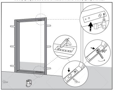
8 Install the hinge at the top and bottom of the door leaf.
