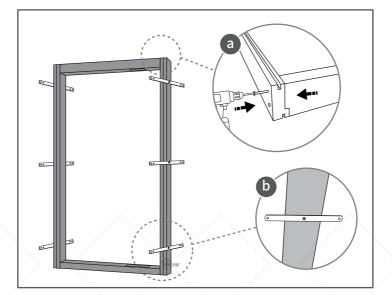
Install the door frame, apply glass glue to the bottom of the door frame at the door opening, and use a level to check if both sides are vertical.
