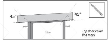
Cut the door cover line, the door cover line opening to fit the gap of the door frame.
